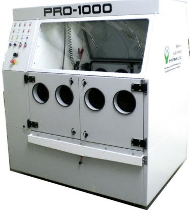
This also allows for 1 to 4 operators the ability to work on the same print at the same time drastically reducing the washing cycle times (although additional pumps will be required to do this) this is particularly useful when the machine is used as part of a production line operation producing very large numbers of small parts at the same time.
